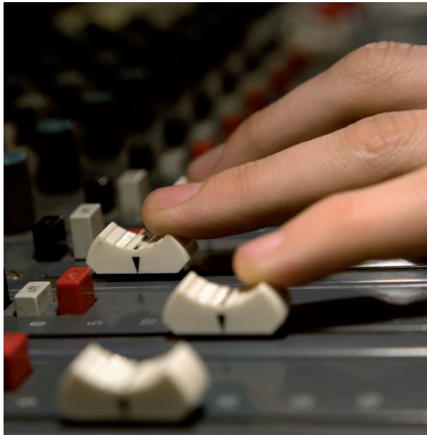
Fig. 1: Traditional faders on a mixing desk give intuitive tactile feedback.
